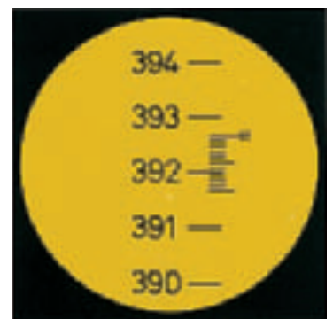
NAK2 circle reading (400 gon) 392.66 gon
